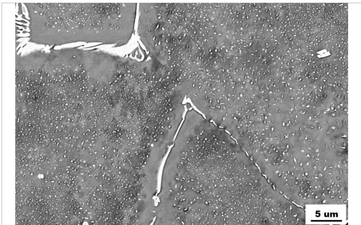
Fig. 1: Fe-28Al-15Si2Mo alloy after HT 800°C/100h. Inside the grains, a large volume of new very fine precipitates formed and were distributed in the form of dispersion.
