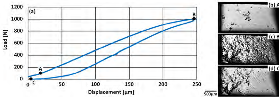
Fig. 1: Load vs. displacement curve of the uniaxial compression test (a) and the in-situ observed microstructures at the beginning (b), at the maximum load (c), and after the end of the test (d).
