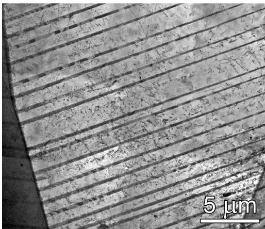
Fig. 1: Mechanical twins formed during cycling, strain amplitude 0.4%, specimen after failure.
