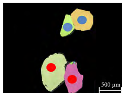
Fig. 2: Agglomerated crystals prepared by chemical transport reaction (preparation method 3)
