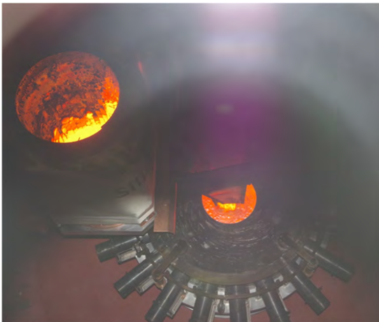
Fig. 1: Induction Skull Melter after pouring
