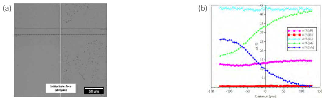
Fig. 1 : Mo/Nb Couple after assembling at 1300 °C for 40 h, (a) SEM-BSE showing the EDS dots and (b) the corresponding concentration profiles (at.%).
