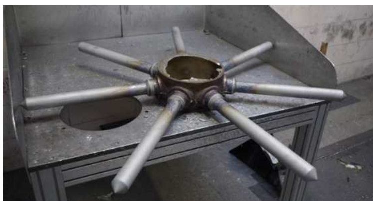
Fig. 1: Centrifugally cast EIGA electrodes for gas atomization
