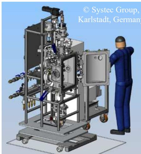
Fig. 1: Design of floating zone furnace
