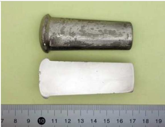
Fig. 1: Appearance and polished cross section of a cylinder-shape ( $d \geq 20 \text{ mm}$ ) MoSiBTiC ingot produced by drop casting under arc melting.
