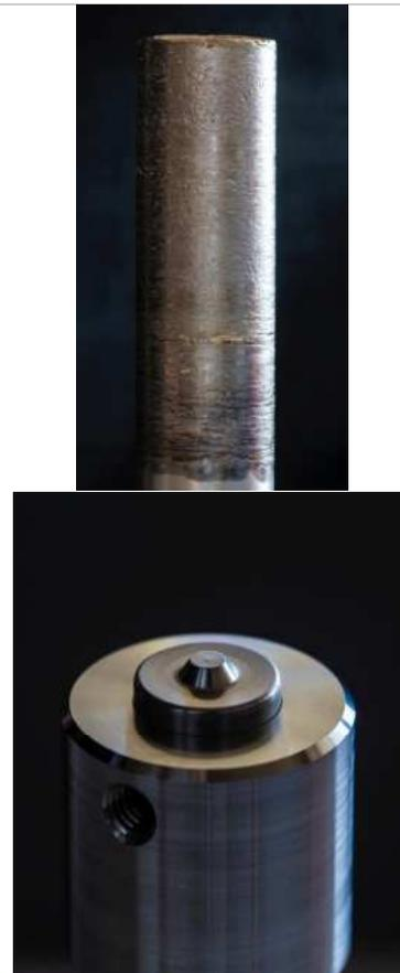
Fig. 2: Appearance of (left) a cylinder-shape ( $d \approx 40 \text{ mm}$ ) MoSiBTiC ingot produced by plasma-melting with a water-cooled pulling-down Cu mold and (right) a work tool of the MoSiBTiC alloy for FSW.
