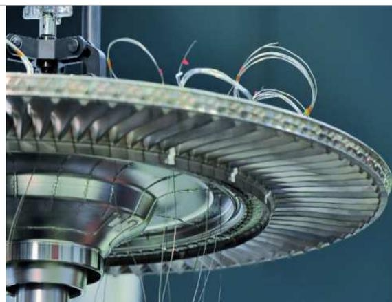
Figure 2: Low-pressure blade assembly of the geared turbofan instrumented for testing
